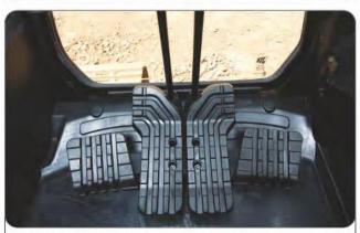
Rubber- coated track pedal and foot rests for operator comfort. Front lower glass can be removed for ventilation.
