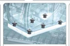
Cabin is mounted on 6 viscous mounts to absorb vibrations.
