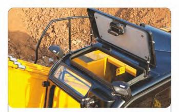
Roof hatch provided to keep the cab well ventilated, which is aided by rear sliding window.
